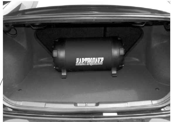
In a hatchback: the tube should lay parallel to the rear of the vehicle, firing into the corners.
